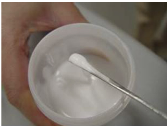
Fig. 3. Appearance of manual deaggregation process of un-wet mass of powder by a small spatula.
